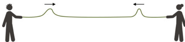
Figure 3.2 Two people putting pulses into a rope that travel toward each other.
